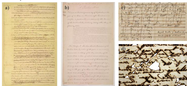
Figure 1. Hand-written materials of iron gall inks a) original draft of the Declaration of Independence; b) Abraham Lincoln's first draft of the Emancipation Proclamation; c) Beethoven's original scores; d) a manuscript with "ink burnt" phenomena which were caused by the high acidity of iron gal ink
